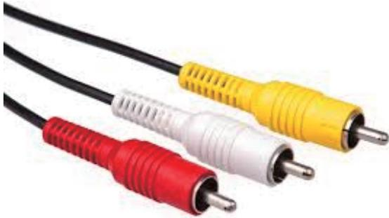
The RCA is the most common connector type on consumer gear for composite and component video, as well as for both digital and analog audio. RCA jacks color-coded yellow on a device usually are composite video inputs and outputs. The RCA connector is not a 75 Ohm design but it is used in a multitude of 75 Ohm applications.
