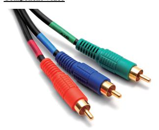
Component video ordinarily refers to "Y/Pb/Pr" or "YUV" video. In Y/Pb/Pr Component Video, there is a luminance channel, "Y", which carries the luminance along with the sync pulses, and two color-difference channels, which carry signals representing Blue minus Luminance (B-Y, or Pb) and Red minus Luminance (R-Y, or Pr). Component YUV separates color and brightness information into three signals, which keeps the color
