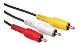
The RCA is the most common connector type on consumer gear for composite and component video, as well as for both digital and analog audio. RCA jacks color-coded yellow on a device usually are composite video inputs and outputs. The RCA connector is not a 75 Ohm design but it is used in a multitude of 75 Ohm applications.
